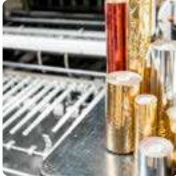
Hot Foil Stamping A metallic or colored foil decorating process on paper, paperboard, leather, vinyl, linen and other materials
