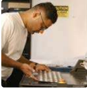
UV Printing A unique method of digital printing utilizing ultraviolet (UV) light to dry and cure the ink upon contact.
